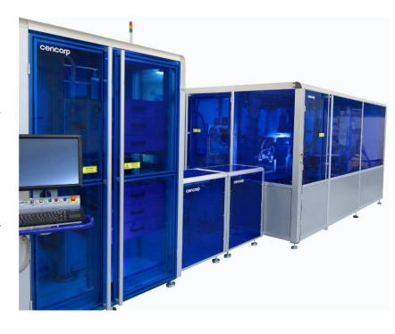
A **Viscotec dispensing** solution makes sure that deposition is made correctly. The **Cognex 8402** verifies that the material is distributed as defined. A **Weber screw driving solution** ensures that tightening is executed according tightest specifications and controls. Final tested products are labeled with **Cab Hermes printer** and print quality is verified with **Keyence SR-710 reader**. Process states are followed by **Omron V680S RFID** technologies and mastered by **NXT7 PLC** platform
